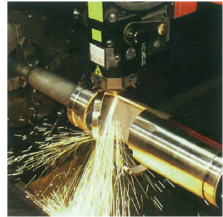
Hunter Innovations uses advanced laser-etching technology to cut passages in stainless steel piping that will accept the backflow-prevention components.
