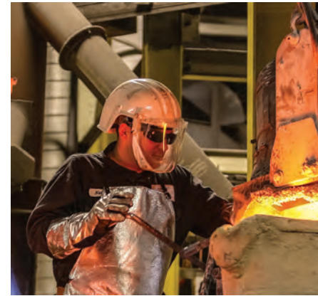
A foundry worker pours liquid bronze into molds.
