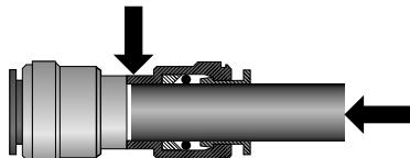
Pull on the tube to check that it is secure. The system must be tested prior to leaving the site and/or before use.
