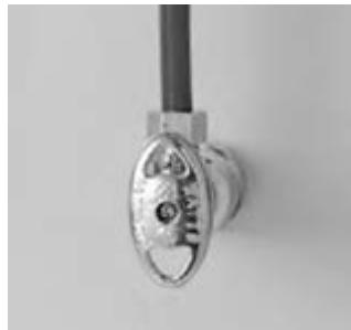
Step 4 - Locate the blue 3/8" tube in the parts bag. Remove a brass nut, plastic delrin sleeve and brass insert from the parts bag. To assemble, place the brass nut on the blue tube first (Open end out), then the sleeve and then push the brass insert all the way into the end of the tube. (See Picture).
