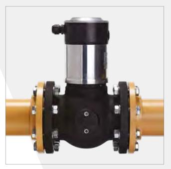
The Powerseat® electro-hydraulic gas shutoff valve allows the control and safety shut-off of low pressure combustible gases in pipes from 40mm to 250mm.
