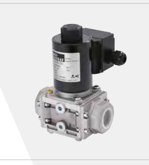
Class A Safety Shut Off Valves, Normally Closed. Gas Families 1, 2 & 3. Cast Aluminium Bodies. Closure within 1 sec. of power being removed.
