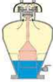
RELEASING AIR UNDER PRESSURE
