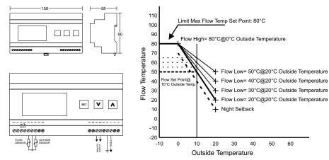
Sensor cables should be screened cable 7/0.2mm max length 100m with the screen earthed at the controller end only.
