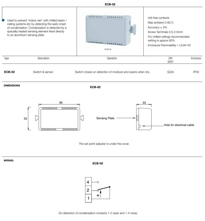
**INSTALLATION:** The unit should be mounted directly onto the coldest part of the pipe/beam.
