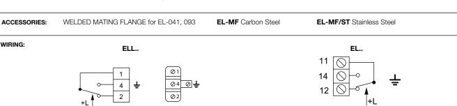
On level rise contacts 1-4 close 1-2 open. On level fall contacts 1-2 close 1-4 open.
