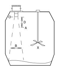
O : Origin of measurement. All measurements (distances / depths) are taken from O.
