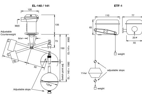
When float reaches upper adj stop C-NC close : When float reaches lower adj stop C-NO close EL-140/141 - The counter balance/weight on the arm/lever should be adjusted for correct operation.
