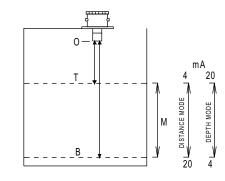
The unit can be set to read in either Distance or Depth mode.M : minimum distance between set points must be > 100mmD : 500mm Dead bandO : Start of measurement
