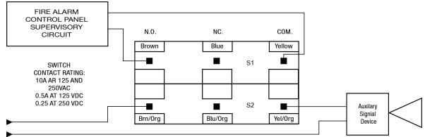
Switch 1: 2 leads per terminal Switch 2: 1 lead per terminal
